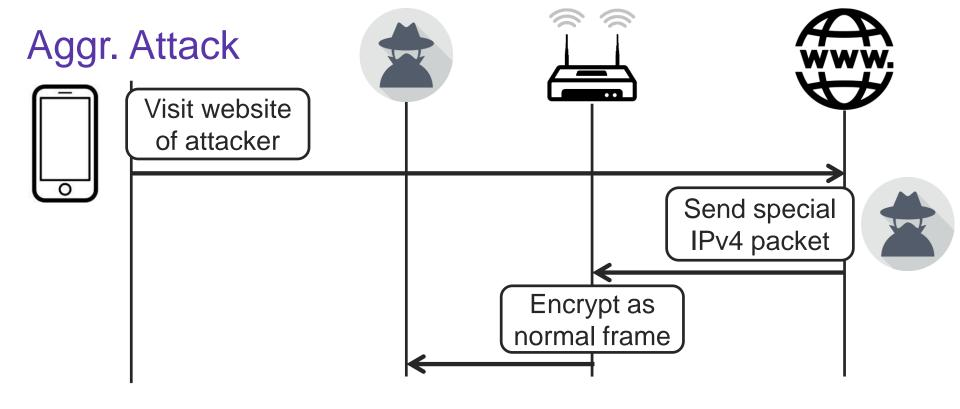
The AP will encrypt the special IPv4 packet and sent it to the client... but the attacker will intercept it first!
