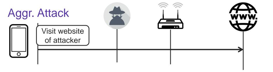
Step 1: victim is tricked into connect to the attacker's server, for instance by visiting their website. This causes the victim to create a TCP connection with the attacker's server.
