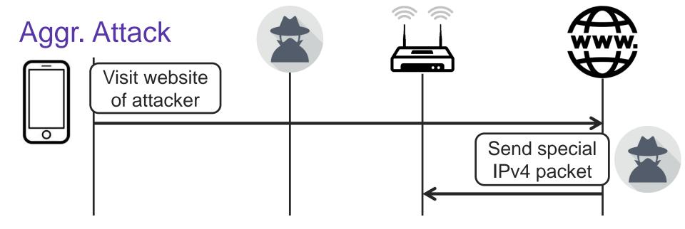
Step 2: the attacker's server sends a special IPv4 packet to the client over this TCP connection.
