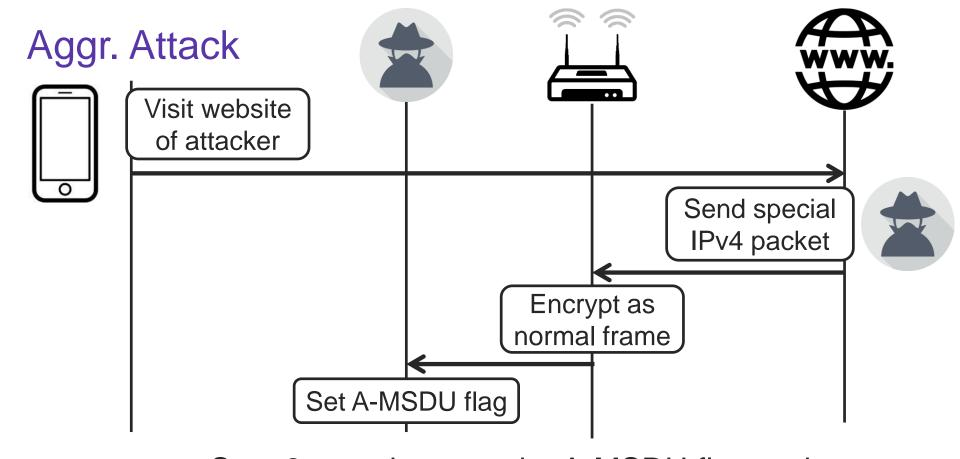
Step 3: attacker sets the A-MSDU flag and then forwards the encrypted Wi-Fi frame.
