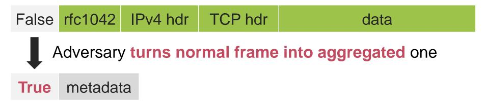
> Metadata = rfc1042 & IPv4 hdr → 1<sup>st</sup> sub-packet is ignored
