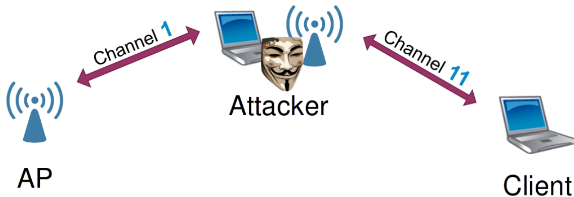
Figure 6: Graphical illustration of a channel-based MitM attack.
